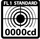
**Peak beam intensity** – The brightest point in the beam measured in candela. Candela is the modern unit of measure for light intensity replacing the now-obsolete unit known as candlepower.
