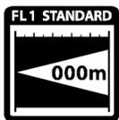
**Beam distance** – The distance, measured in meters, at which the light projects a useful amount of light, measured at 0.25 lux. (0.25 lux is approximately the equivalent of light emitted from a full moon “on a clear night in an open field.”)
