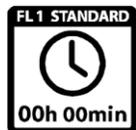
**Run time** – Tested with fresh batteries from 30 seconds after the light is turned on until the light output reaches 10% of the initial measurement. This is the total time of useable light before most consumers will change batteries.
