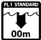
**Water Proof** – Water submersion depth rating, measured in meters. This icon indicates at least an IPX7 rating which means the sample is submerged to a minimum of 1 meter depth for 30 minutes. If this test is performed, it must be done after impact resistance testing is completed to ensure water tightness under real-life conditions.
